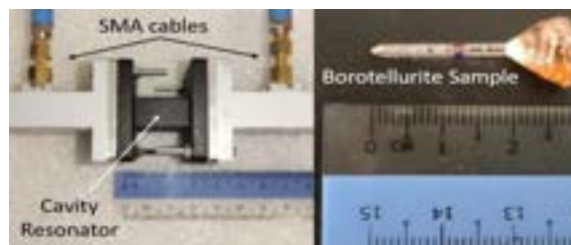
Figure 2. Rectangular cavity resonator (left) and borotellurite sample (right).
